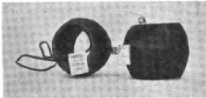
Fig. 2.—H.F. Auto-transformers. Left: 2,000 turns 28 S.W.G. enamelled copper. Right: 2,000 turns 26 S.W.G. enamelled copper. Internal diameter 2 1/4".
