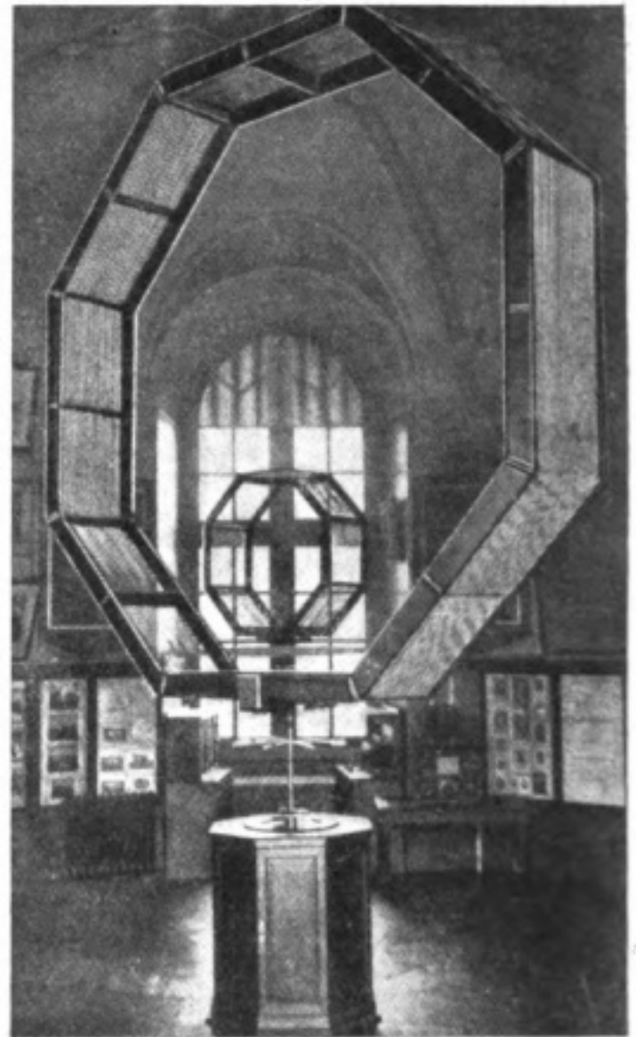
Installation at the Paris Observatory for the comparison of Time Signals received from Eiffel Tower, Lyons, Bordeaux, Annapolis, Nauen and other stations with the pendulum of the Observatory clock. Signals received on the frame aerial shown in the photograph are thus compared by aural methods and by self-registering apparatus shown near the window.
