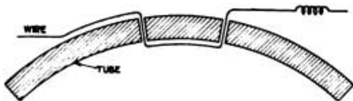
Fig. 4. Method of passing wires through the tube.
